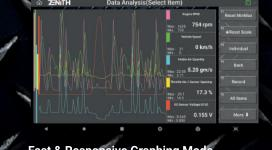
Fast & Responsive Graphing Mode Z5 offers fast yet intuitive graphing mode which instantly self-adjusts maximum and minimum scale; enabling the users to more accurately observe and compare live data.
