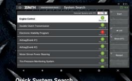
**Quick System Search** 'System Search' option automatically scans all the vehicle systems, reports fault codes, and provides access to advanced diagnostic functions in each detected systems.
